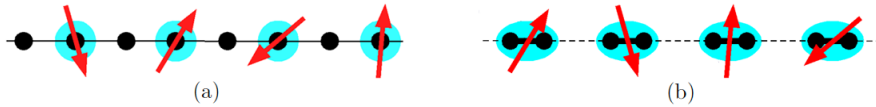
Fig. 1. Two characteristic insulating state in the quarter-filled bands depending on the degree of dimerization; charge ordering (a) or dimer Mott (b) for weak or strong dimerization, respectively.
